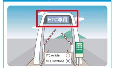
The system detects when a vehicle is in the lane and the bar opens. Pass through the gate only after you are sure the bar has opened. Ensure to reduce your speed, and do not brake suddenly just in front of the bar, as this risks causing a collision!
